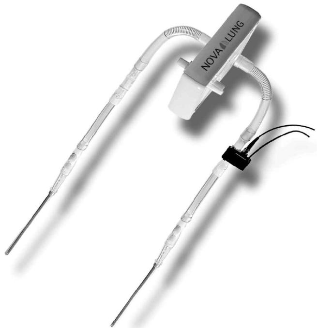
Figure 2 The symmetrical lung assist device is shown with two low resistance cannulae attached. The system's low pressure gradient allows use without a mechanical blood pump in an arteriovenous shunt created between femoral artery and vein.
